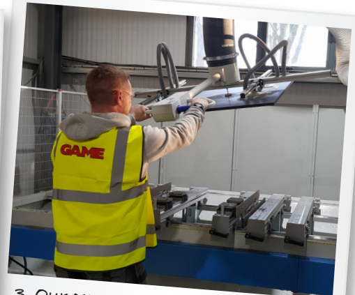
3. Our compressed air lifting machine then lifts the cut TRESPA® onto the Masterwood Project 250 CNC
