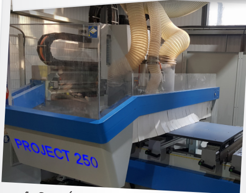
4. Once in place, the machine cuts all the shapes, holes and finishes into the TRESPA® - accurate to 1/10th of a millimetre
